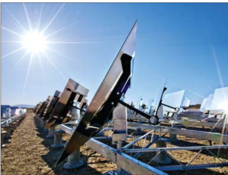
Concentrating solar thermal power with heat storage can provide reliable electricity even when the sun isn’t shining.
