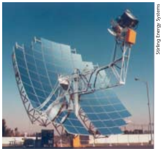
Stirling solar dishes efficiently transform solar heat into electricity.
